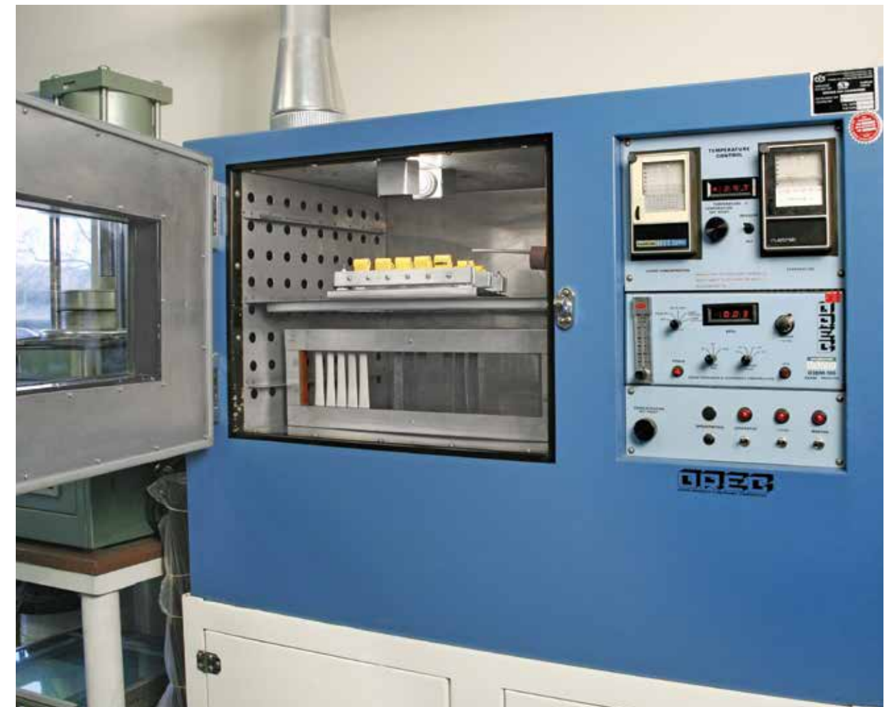
Quality control lab testing in our Ozone exposure chamber
