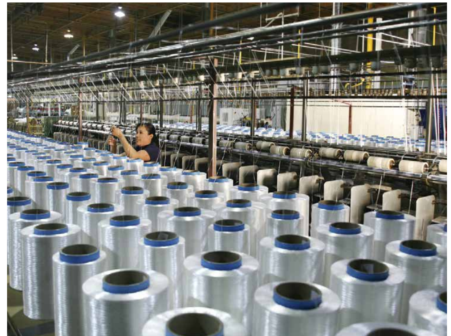
The ring twister combines multiple plies of high tenacity filament polyester yarns.
