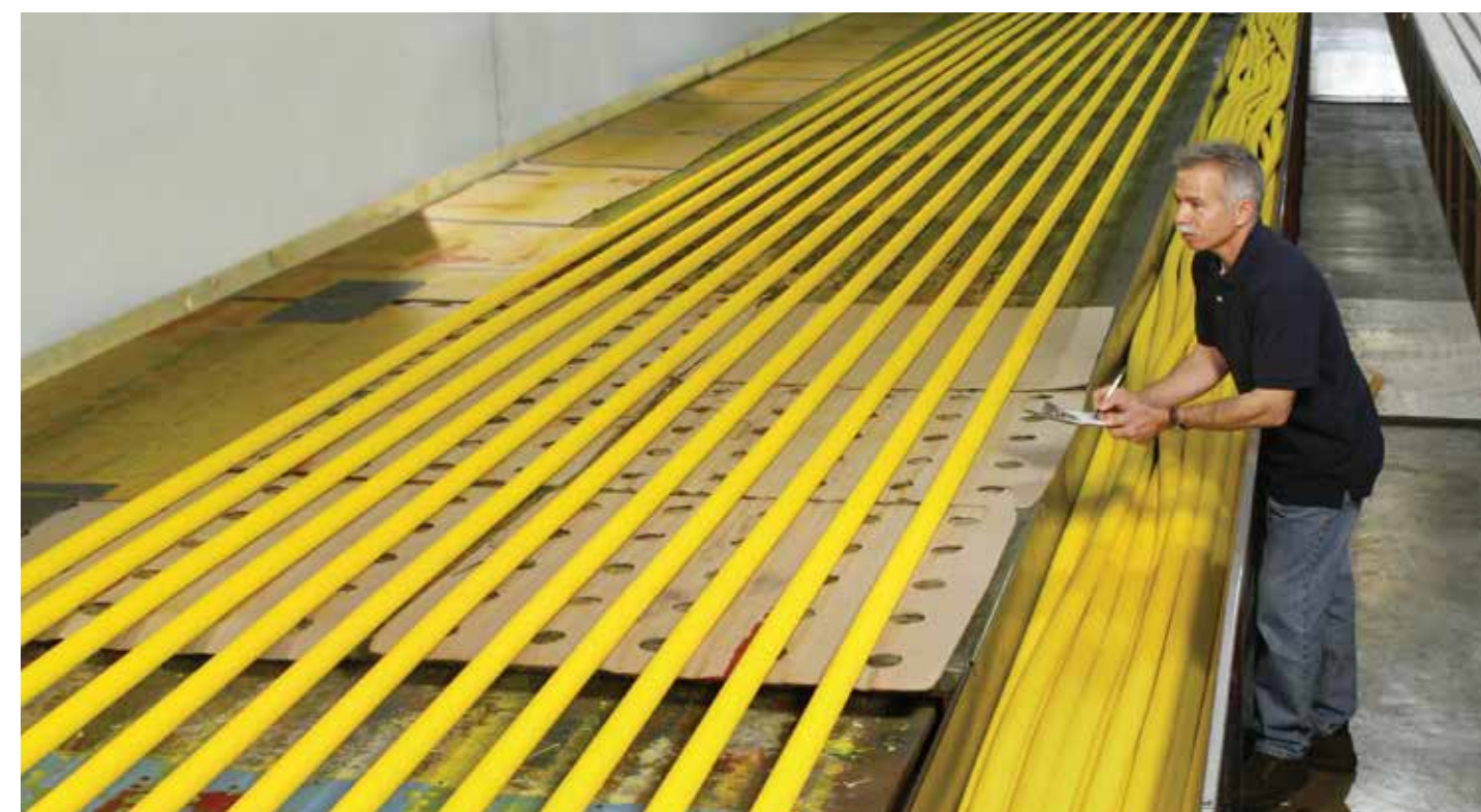
Curing Process for Dura-Bond™ Vulcanized Adhesion System
